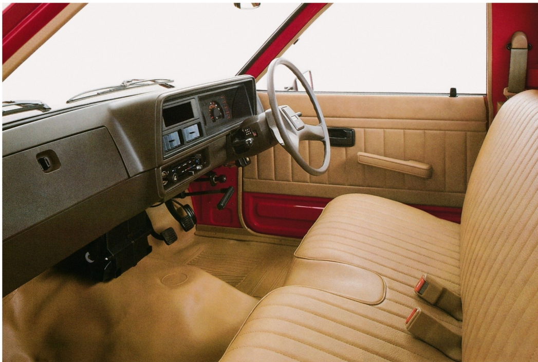
Above: The spacious KB 26 three-man cab. The KB 41 cab is identical, except for its floor-change gear levers.
