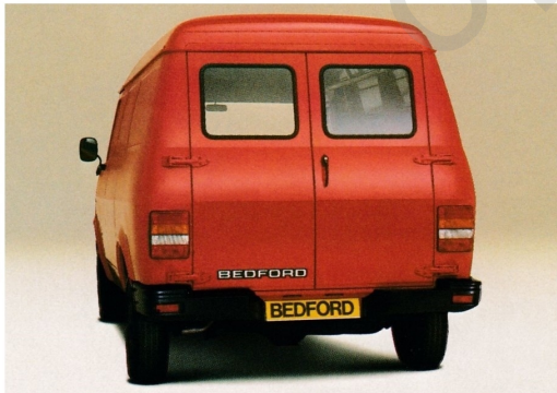
Right: All CFs have wide, side-hinged rear doors. Long wheelbase models (CF280 shown) have increased roof height.
